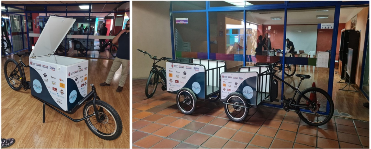
Fig 1. Locally assembled e-cargo bikes, long john type (left), rear-load and front-load tricycles (right)
